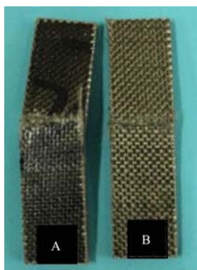
注：A 为老化弯曲试件，B 为老化后弯曲试件。 Note: A is bending specimens before aging, B is bending specimens after aging.
